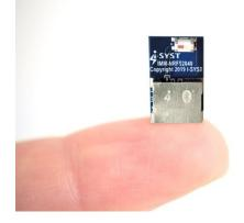
The **IMM-NRF52840** SoM is built around the Nordic Semiconductor ultra low power nRF52840 32-bit ARM<sup>®</sup> Cortex<sup>™</sup> M4F CPU with floating point unit running at 64 MHz. It integrates the nRF52 series 2.4GHz transceiver with programmable output power -20dBm to +8 dBm, USB 2.0, Flash memory, analog and digital
