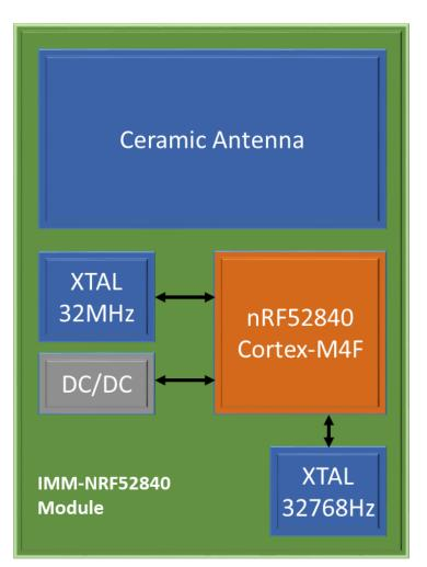
Figure 1: Module internal diagram
