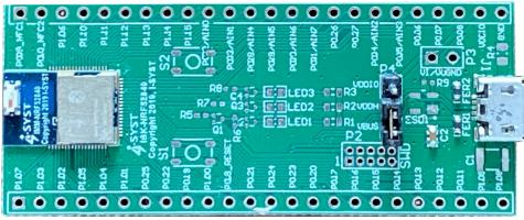
Figure 5: IBK-NRF52840 Breakout Board.
