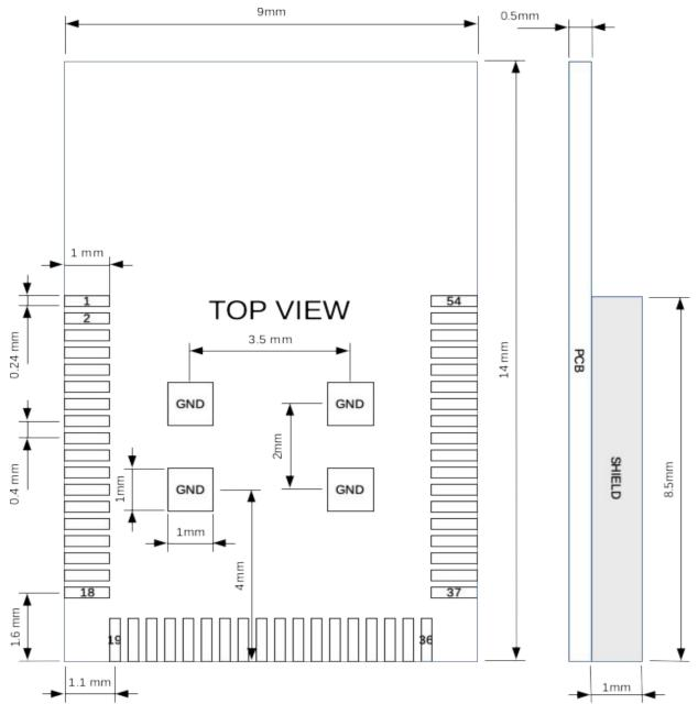
Figure 2: Dimensions top view
